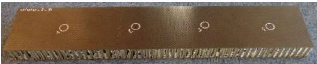
Figure 17.7 - SDOF SAS panel of 50mm in thickness
