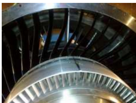
Figure 17.11 - Straightener blades with 30° inclination in the direction of rotation
