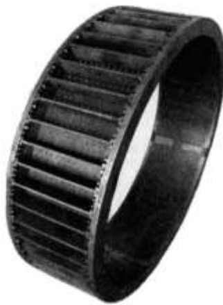
Figure 17.8 - View of latticed suppressor in flowpath section of stage C179-1
