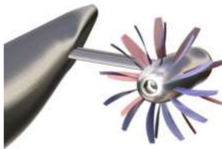
Figure 17.9 - 3D model of open rotor under researching
