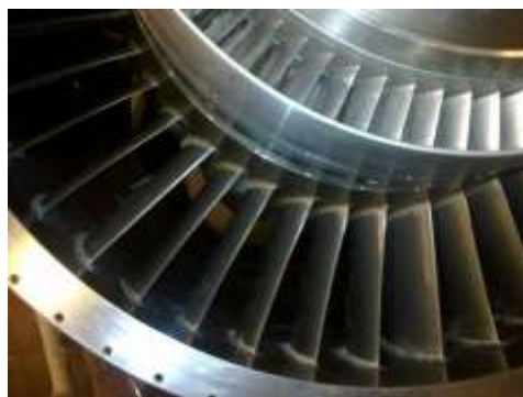
Figure 17.10 - Straightener blades without inclination
