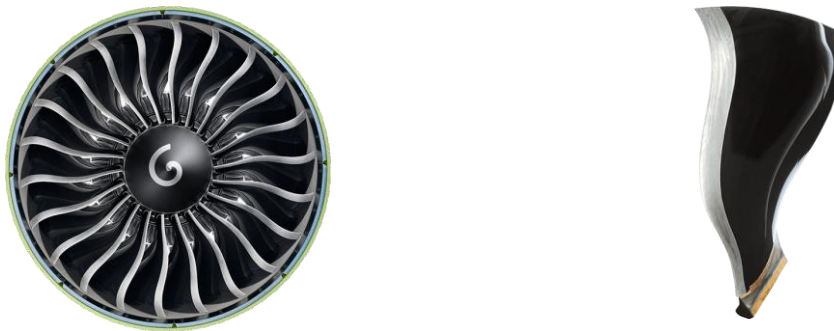
Figure 13-A.34. Fan and blade of engine GE90-115B
