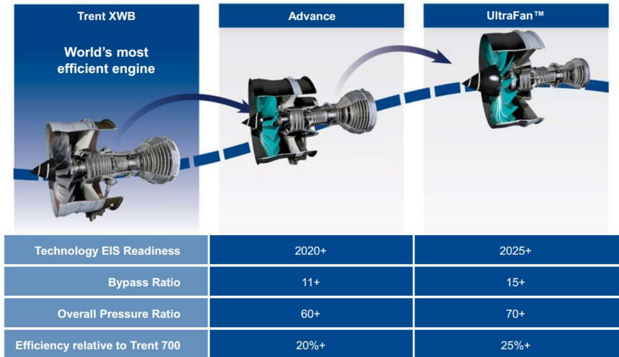
Figure 13.88. Comparison of modern Rolls-Royce engines with Advance and UltraFan.
