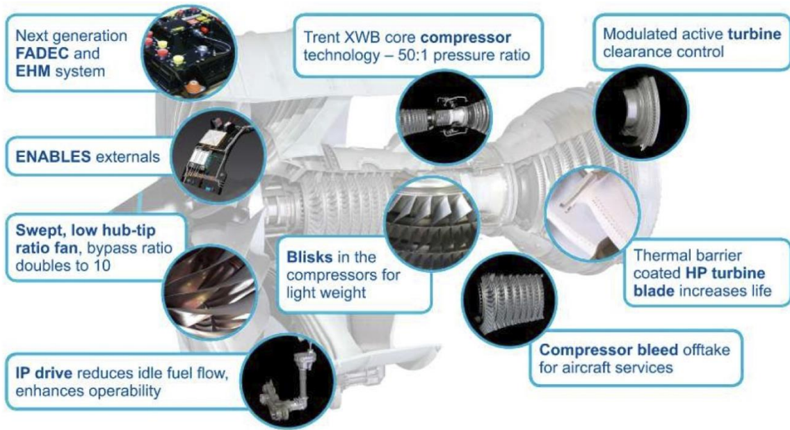
Figure 13-A.44. Features of engine Rolls Royce Trent 7000
