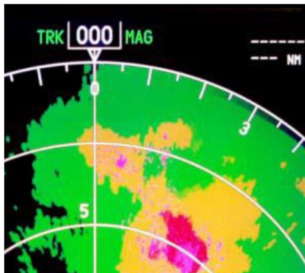
Figure 5.45 - Cockpit radar display of turbulence [16]
