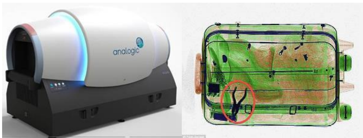
Figure 5.74 – Computer tomography scanning creates 3-Dimension Image
